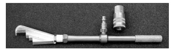
This model has been made for several years now and is becoming very popular with engineers wanting a <u>light</u> pitot tube. The handle part is machined from a solid piece of brass, allowing it to be both skinny and very strong. It is still easy to hold on to with its knurled handle. *We recommend this model with any of the ultra-thin blades*.
