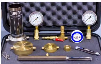
**#805 All Purpose Test Kit:** Includes all of our most popular items. #101 quick disconnect pitot tube with #108 spare blade, 2 of the #202 Custom Model liquid filled gauge (2 ½" Dial), #501 inspector's hydrant flow nozzle, #404 double ball valve quick disconnect bleeder, #301 brass hydrant test cap, #303 brass hose cap, #304 brass faucet test cap and #905 Plano large All Weather Case. **\$465.00**
